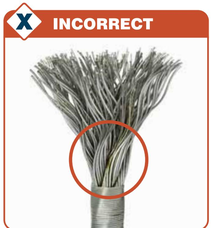
Figure 4: Incorrectly broomed wire rope.
