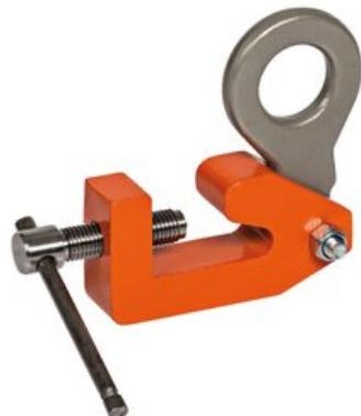
**General:** For use as a temporary lifting point in any room where HP-profile is being used, such as sectional ship parts and ship engine rooms. The BSW clamp is equipped with a thread spindle for attaching the clamp. The clamp is used for HP-100 to HP-240 (HP = Hollandprofile)
