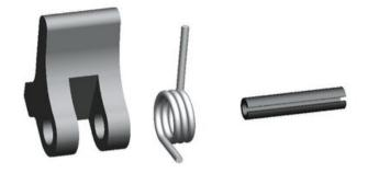
Trigger sets for LHW, KLHW and WLH(B)W safety hooks consist of a high-strength safety lever, a spring made from rust-proof spring steel and a retaining pin. The sets come with auxiliary material to facilitate assembly as well as detailed assembly instructions to make sure that your safety standards leave nothing to be desired.
