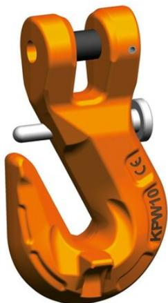
KPSW Clevis grab hook with safety catch against accidental release of the chain. Designed for the mounting of chain slings. For shortening and for slings that must not tighten. Reduction of load capacity not required thanks to 4-fold safety.
