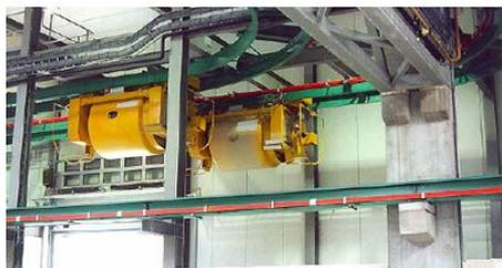
**General:** AKAPP Multiconductor system has a unique concept. Based on free expansion of housing and conductors. Due to the absence of plug connectors, the conductors offer the most reliable transmission of energy and signals. The ideal conductor system for cranes, conveyors, automated warehouses and many other applications
