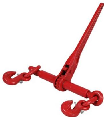
The Green Pin® Ratchet Loadbinder HK EN12195-3 is a ratchet type loadbinder with hooks according to EN 12195-3. The ratchet of this loadbinder enables the precise setting of the lashing length and tension. The loadbinder is also equipped with a safety latch that prevents the chain from sliding back. The Green Pin® Ratchet Loadbinder HK EN12195-3 is available in a range to suit 8 mm up to 16 mm grade 8 chain.
