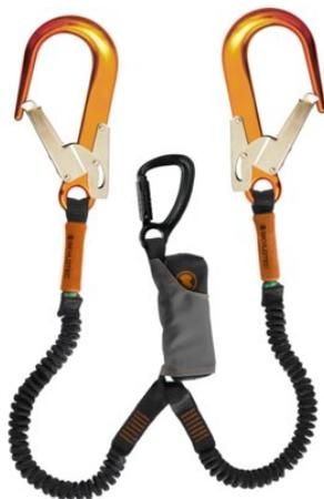
Revolutionary, patented energy absorber with the large weight range from 50 kg to 140 kg which always withstands a maximum impact of less than 6 kN at a maximum absorber length of 1,75 m. Meets the most international standards in one single product.
